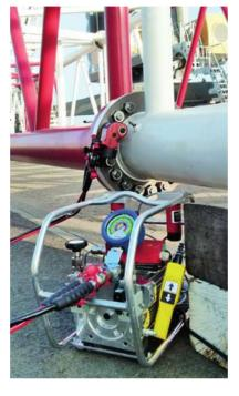
Fast and easy one-man operation by the remote of the hydraulic pump Hydro-DAX 18.
