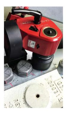
A handle-bar can be mounted on and off the housing of the CX easily for an easier handling.
