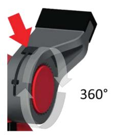
The reaction arm can be adjusted in 360° along the splined housing. The asymmetrical design allows set-up of the reaction arm in both directions.
